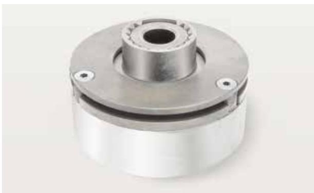
Servo drives require low-backlash holding brakes with short operating times. With its temperature-resistant friction lining, the BFK417 is ideally equipped for emergency stops even at high speeds. This makes it a cost-effective alternative to the permanent magnet brake.
